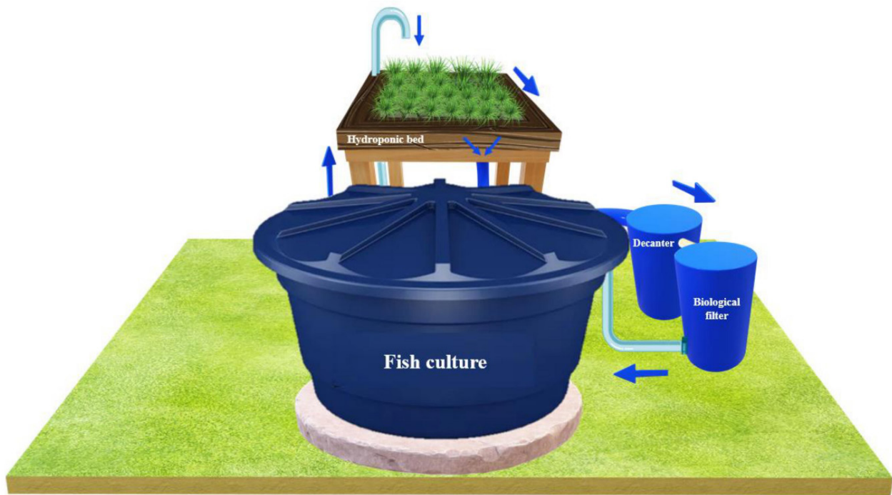
Figure 1: Graphical representation of independent aquaponic systems used for integrated culture of tambaqui C. macropomum with açai E. oleracea for 180 days. Each aquaponic system consisted of a 1,000 L (800 L useful) circular polyethylene tank for fish, with a 70 L decanter, a 100 L biofilter, a pump (3000 L h -1 ) for water recirculation in the system and a 150 L cultivation bed for açai seedlings. The figure was designed by the authors using Microsoft® PowerPoint program.
