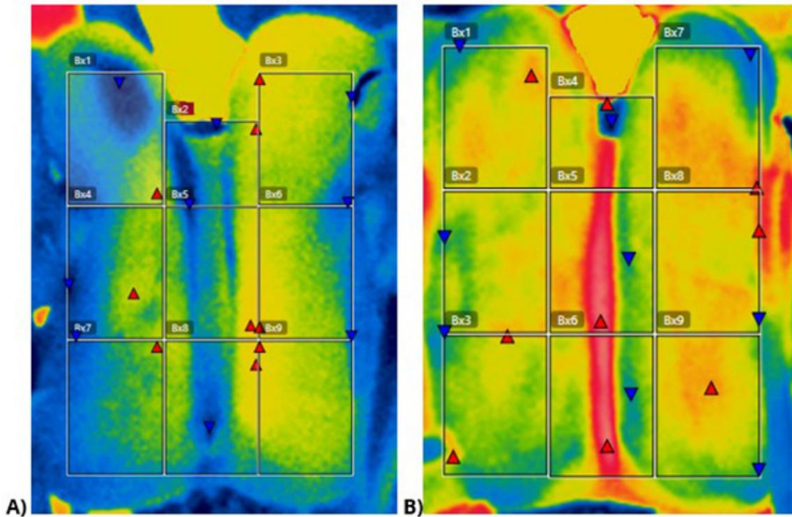
**Figure 2:** Thermographic image of the ventral face of the Australian saddle before (A) and after (B) its use in a basic horseback riding course
