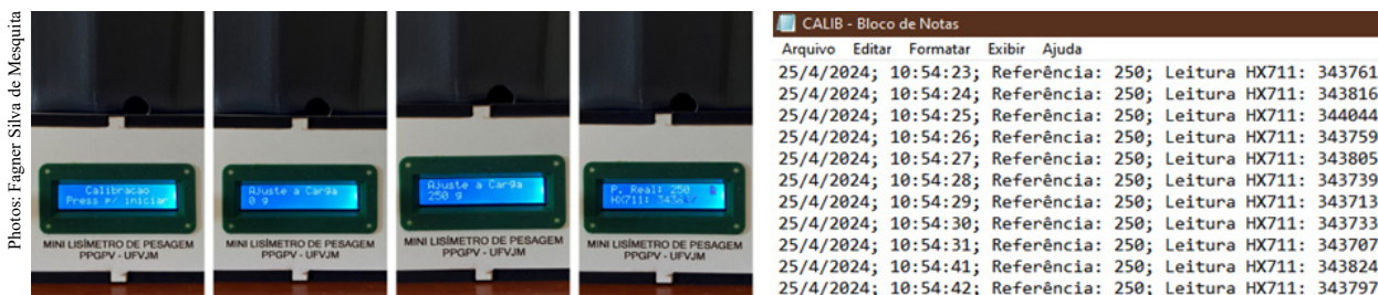
Figure 4. System calibration - standard weights, HX711 readings, and LCD records.
