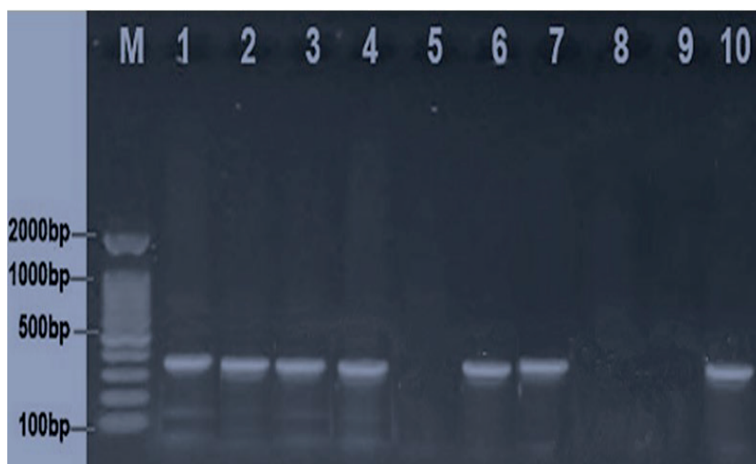
Figure 2. An agarose gel electrophoresis image that shows the PCR product analysis of the Helicobacter pylori cagA gene with 349 bp PCR product size.
